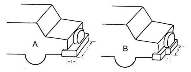
There are two styles of continental kits, one where the rear bumper has been extended over its full width (style "A"), and the other, where the bumper has been extended at the area of the continental kit only (style "B").
